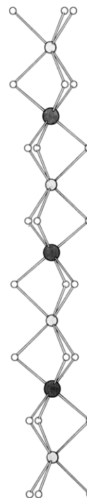
Figure 2. Single chain in the Sr 3 NiPtO 6 structure: platinum (large shaded circles), nickel (small shaded circles), oxygen (open circles). The alternating PtO 6 and NiO 6 polyhedra have local O_h and D_{3h} site symmetry, respectively.
